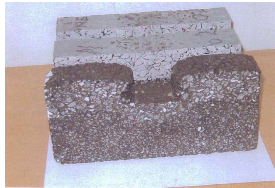
Cross section of three specimens after 20.000 passes. In front asphalt wearing course on low grade asphalt, second Densiphalt on low grade asphalt, in the back reinforced Densiphalt on low grade asphalt.
