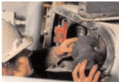
Figure 10. Installation of wear-resistant Densit® end screw in powder pump.
