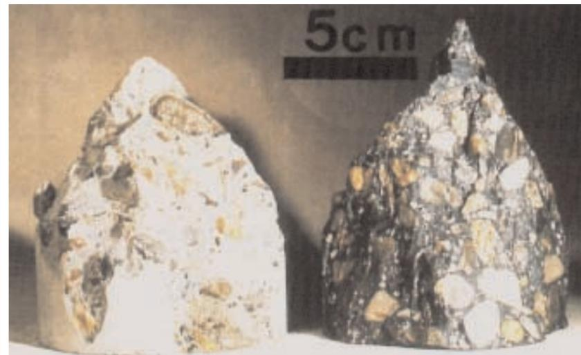
Figure 5. Crushed test samples of ordinary concrete (left) and Densit® (right).
