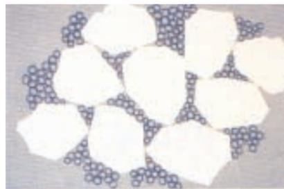
Figure 4. Packing of cement grains and microsilica in Densit®.
