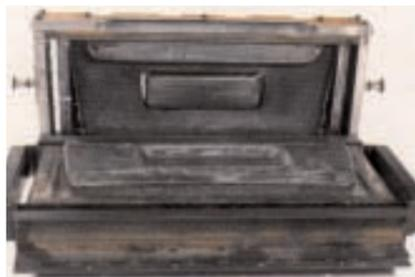
Figure 11. Thin sheet form tool made of Densit®.
