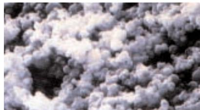
Figure 3. Electron microscopy of microsilica.
