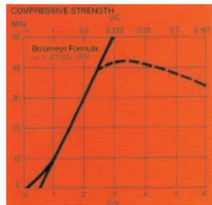
Figure 1. Compressive strength of conventional concrete as a function of the water-cementitious material ratio.
