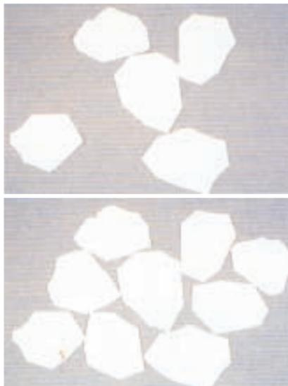
Figure 2. Packing of cement grains in conventional concrete – without (top) and with (bottom) superplasticizing admixtures.
