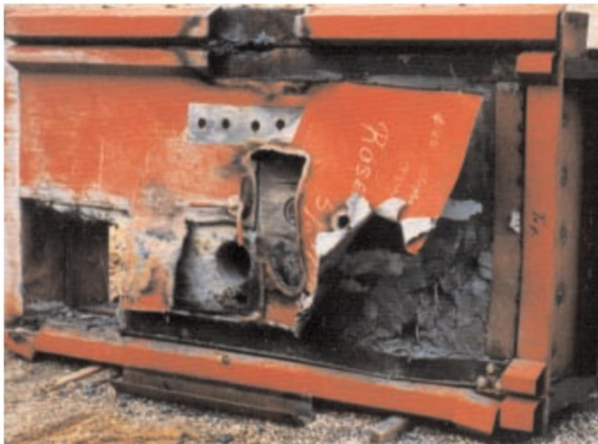
Figure 15. Safe constructed in Densit® following a successful test. The material is used today by a majority of the leading safe manufacturers in Europe.
